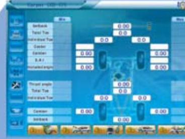
Measured Screen Helping decide how to adjust by showing whole condition with measured each values
