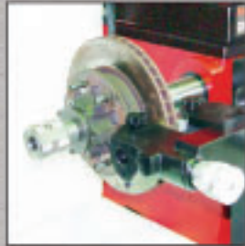
Resurfacing of hub disks
